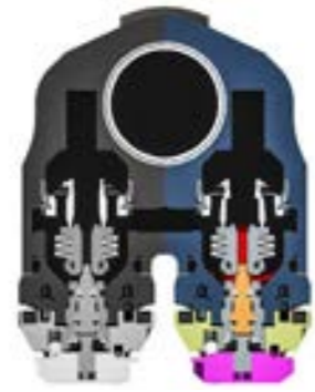
OILFLOW COMPRESSION LOWSPEED
