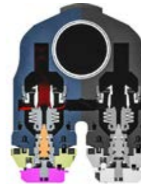
OILFLOW REBOUND LOWSPEED CLOSED
