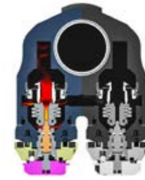
OILFLOW REBOUND HIGHSPEED
