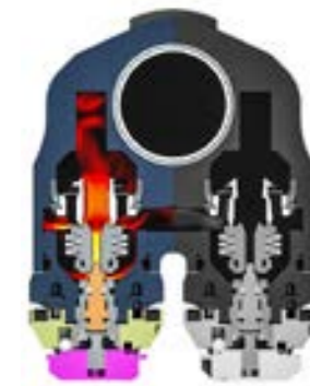
OILFLOW REBOUND BLOW OFF
