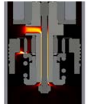
OIL FLOW AT OPENED REBOUND STAGE
